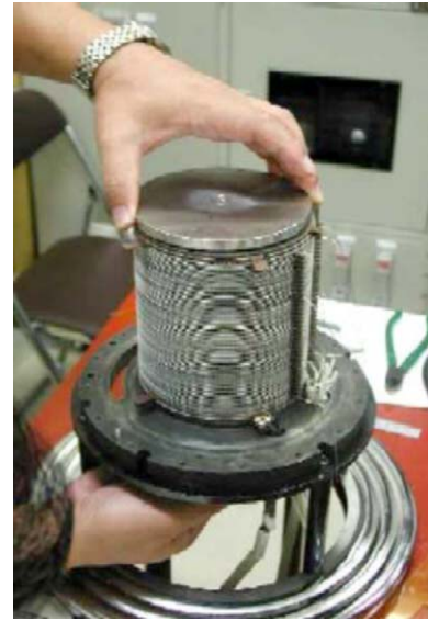
Fig. 1. Planar type 1 kW SOFC stack with 68 cells prepared for 1 kW SOFC system.
