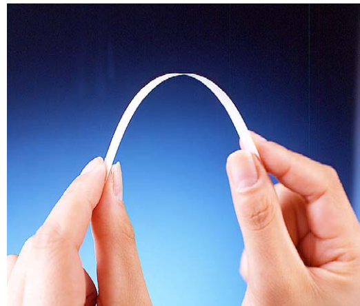
Fig. 3. Flexible scandia stabilized zirconia (ScSZ) ceramics sheet with a composition of 4 mol % \text{Sc}_2\text{O}_3\text{-96 mol % ZrO}_2 .
